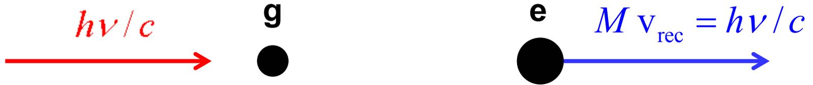
The atom, in the ground state  $g$ , absorbs a photon with momentum  $h\nu/c$ . It jumps to the excited state  $e$  and gains this momentum  $h\nu/c$ . It recoils with a velocity  $v_{\text{rec}} = h\nu / Mc$ .
