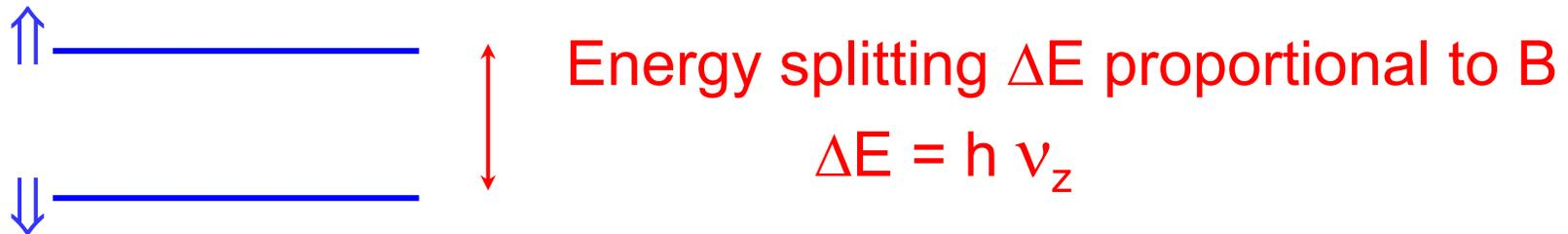
Magnetic resonance : transitions between the 2 spin states induced by a radiofrequency wave with frequency  $\nu_z$
